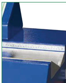
▲ BASE APPOGGIATUBO AUTOCENTRANTE SELF-CENTERING HOSE SUPPORT BASE
