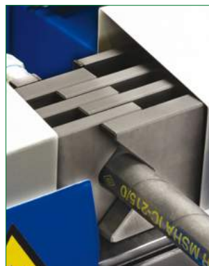
◀ MORSA PNEUMATICA AUTO- CENTRANTE - SELF-CENTERING PNEUMATIC VICE
